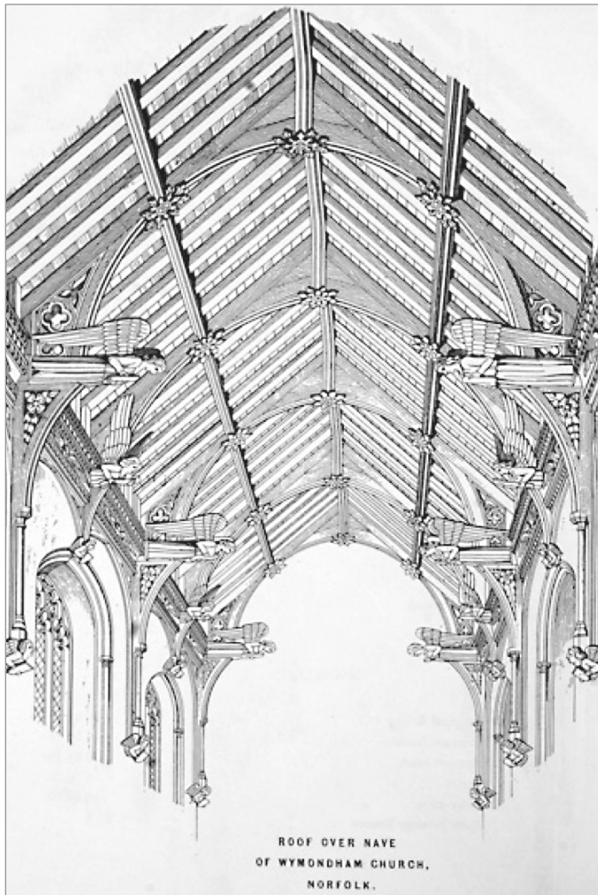
FIG. 28. NORFOLK, WYMONDHAM CHURCH, NAVE ROOF. | RAPHAEL, THE OPEN TIMBER ROOFS OF THE MIDDLE AGES , PL. XX.
